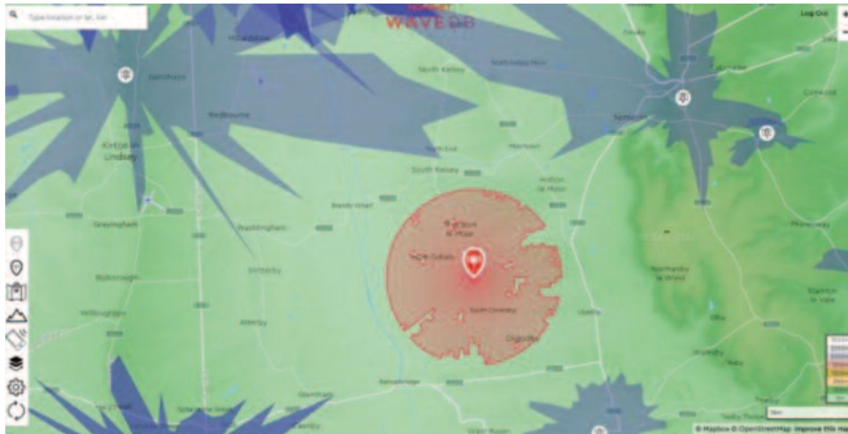
Fig.4 Coverage in-fill from new entrant using the unused spectrum of a licensed MNO
